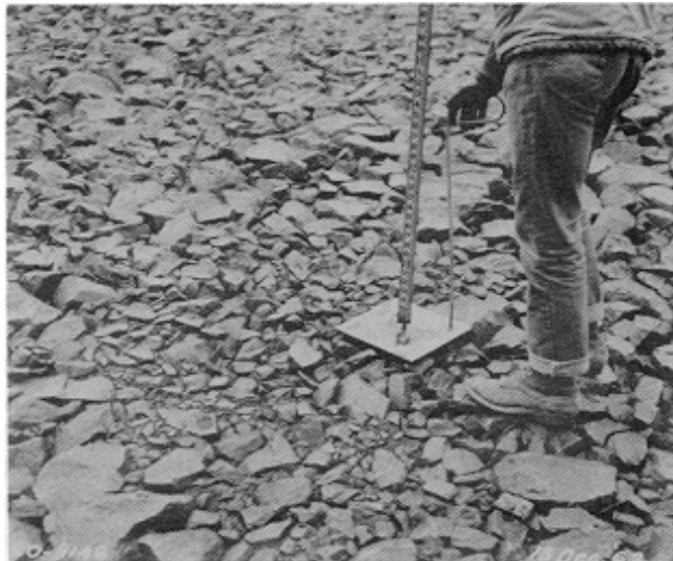
Figure 11-2. Apparatus for taking level readings
